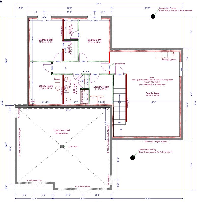
\*2x6 Exterior House Walls - 8'-1 1/8" High \*2x6 Exterior Garage Walls - 10'-2 1/4" High (Verify) \*8" Thick Concrete Basement Walls - 92 7/8" Ceiling \*20" Engineered Floor Trusses (Figured For Elevations) Actual Truss Size May Differ (Verify w/Truss Company) Square Foot Calculations:
